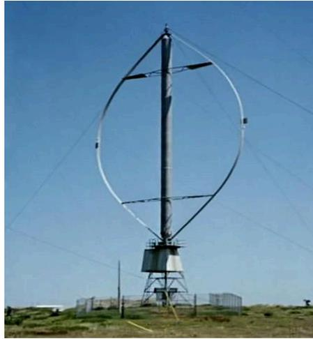
**Figura 10 –Aerogerador vertical**
