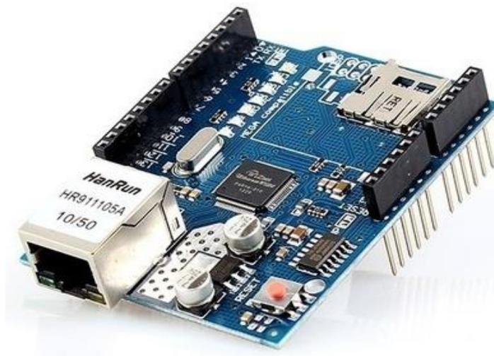
**Figura 5 - Arduino Ethernet Shield**
