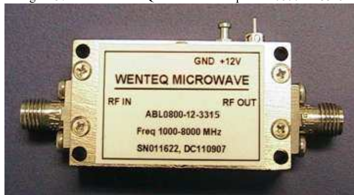
Figura 37: LNA WENTEQ Microwave Corp- ABL0800-12-3315
