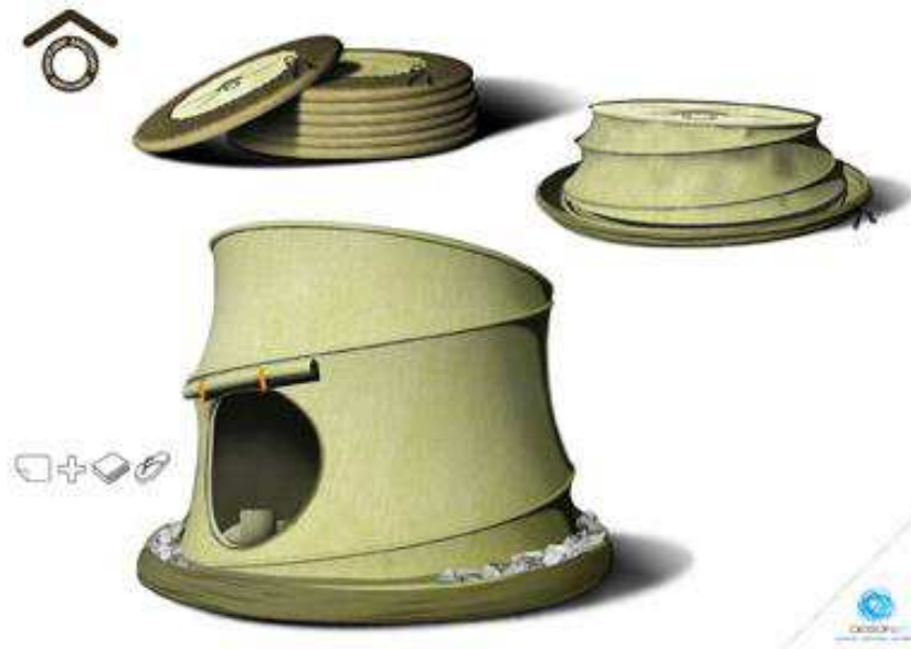
Figura 26: Forma compacta e armada do abrigo emergencial Sanctuary .
