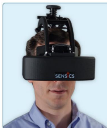
Figura 6. Video see-through (piSight ultrapanorâmico HMD)
