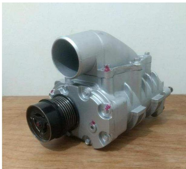
**Figura 4.5. Supercharger EATON M24.**
