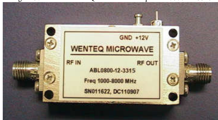
Figura 37: LNA WENTEQ Microwave Corp- ABL0800-12-3315
