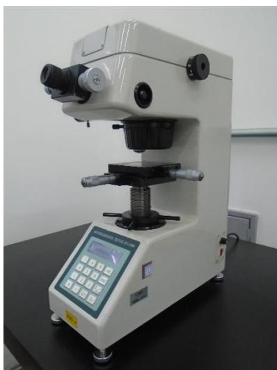
Figura 4.12 - Micro Hardness Tester HV-1000 (Autor)
