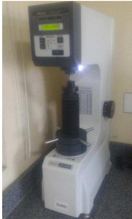
Figura 42 - Durômetro Mitutoyo – HR-430MS. (Autor, 2018).
